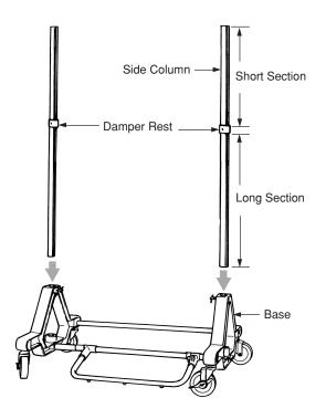
Pit the damper onto the side columns and lower the damper onto the damper rest. Next, secure the damper in its position with the damper wing bolts. At this time, tighten the wing bolts that secure the side column to the base as well.
