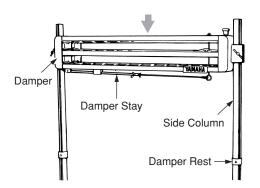
Remove the damper stay, attached to the bottom of the damper, loosen the wing bolt on the damper stay, and attach the stay to the pedal hook. The pedal's position can be controlled by adjusting the length of the pedal stay with its two wing bolts. At this time, tighten the upper wing bolt first, then go on to tighten the lower bolt.
