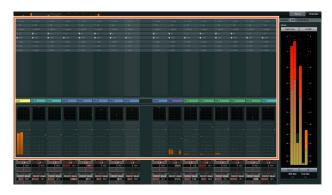
The buttons [QUICK CTRL], [PRE], [ROUTING], [PAN], [SENDS], [CUES], [INSERT], [DYN], and [EQ] are for selecting the "Section" view and the controllable parameters of the [Multi function knobs]. For example, when you press [EQ], the "Section" view changes to the "EQ" view and the controllable parameters of the [Multi function knobs] change to "EQ."
