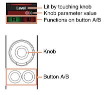
Depending on which controllable parameters are selected in the SECTION CONTROL section, the [Multi function knob] has the following functions.
