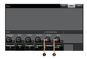
For the buttons used to adjust the pressing time for Smart Switch Delay, the [TALK BACK] button and other buttons can now be configured separately.
