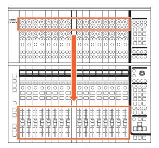
It should be noted that certain parameters assignable to [Multi function knobs] cannot be controlled using the [Faders].
