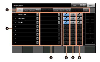
1 Control Room channel selection area Enables you to select the target channel for "Insert."
