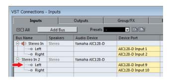
When you assign an input bus which contains multiple channels, such as stereo or surround, to an input channel to control the AD8HR parameters, the parameters of the channel listed on the top of the bus configuration (e.g., "Left" in the case of stereo) displayed in the "VST Connections" window of the Nuendo are displayed. When the parameters of all channels contained in the same bus are not set to the same value, "\*" is added to the end of parameter name (e.g., "HA GAIN\*").
