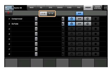
The tab switches between insert slots 1 - 8 and 9 - 16.
