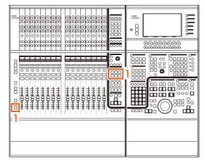
1. While pressing [ALT] in the MODIFIER section, press either [INPUT], [AUDIO], [OUTPUT], [FX], [GROUP], or [OTHERS].
