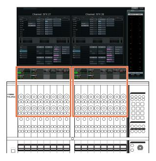
If you again press the [e] button for a channel being edited, the "Mixer" will reappear. It should be noted that, even when Channel Setting mode is active, the specific parameters controlled by the individual [Multi function knobs] can be changed in the SECTION CONTROL section.
