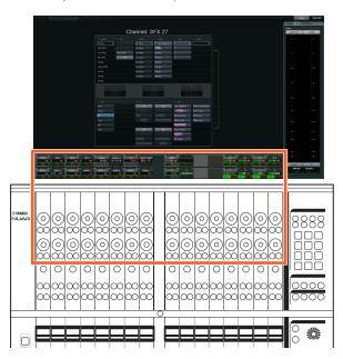
Alternatively, if the [e] buttons for two different channels are pressed at the same time, it will be possible to edit both of those channels simultaneously.
