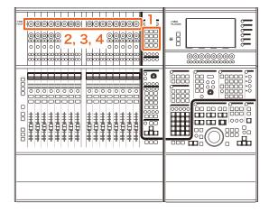
1. Press [VCA] in the SECTION CONTROL section.
