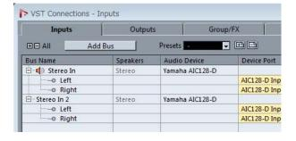
If an input bus with multiple channels (such as stereo or surround channels) has been assigned, the parameters for the bus channel appearing first in Nuendo's "VST Connections" ("Left" for a stereo channel) are shown.
