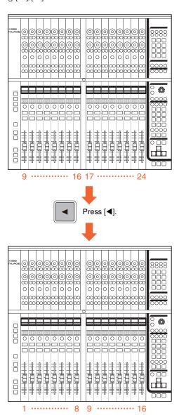
To scroll continuously through the channels, hold down [◄]/[▶]. However, channels in the Left Lock and Right Lock areas cannot be scrolled through.
