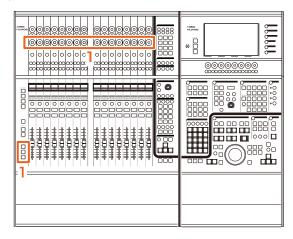
1. While pressing the [SHIFT], [CTRL], and [ALT] keys in the MODIFIER section at the same time, operate a [Multi function knob] (lower).
