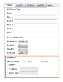
IP address settings for the Nuage Fader and Nuage Master depend on the IP address settings of the MMP1.
