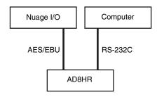
Connect the AD8HR and Nuage I/O by AES/EBU, and connect the AD8HR and a computer by the RS-232C (cross cable).
