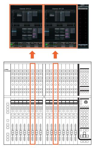
In such a case, 16 of the [Multi function knobs] can be used with each. Of the two channels, the one on the left can be controlled by the left bank of 16 knobs and viceversa.
