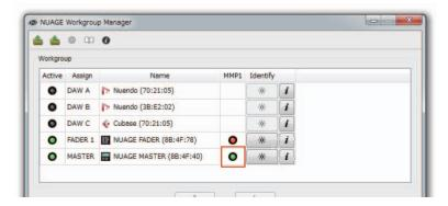
When the MMP1 indicator lights up in red (this means connection failure), the possible causes are as follows:
