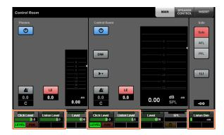
Click Level and Click Pan can be switched using [Multi function button A] and [Multi function button B].
