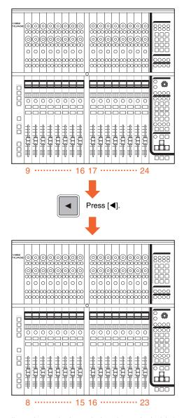
To scroll continuously through the channels, hold down [◀]. However, channels in the Left Lock and Right Lock areas cannot be scrolled through.
