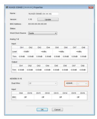
The AD8HR can also be set up in NUAGE HA Remote Setup. To open NUAGE HA Remote Setup, click the Nuendo menu "Devices" → "NUAGE HA Remote Setup."
