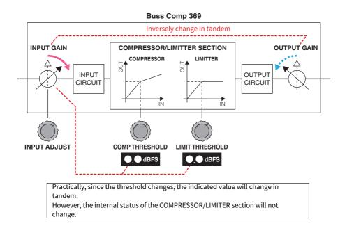
Practically, since the threshold changes, the indicated value will change in tandem. However, the internal status of the , COMPRESSOR/LIMITER section will not change.
