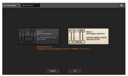
This window allows you to switch the routing mode for HY slot 2.
