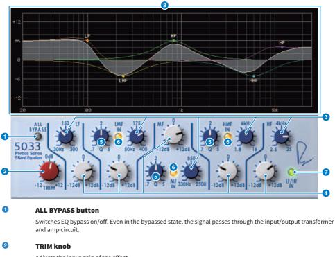
Adjusts the input gain of the effect.
