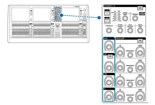
CH Parameter > Controlling GAIN via the Selected Channel section (CS-R5, CS-R3)
