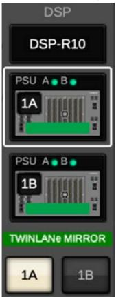
For a DSP Mirroring configuration, a button for switching the DSP engine between active/standby and DSP popup buttons for two units are displayed. In this case, the SYSTEM CONFIG [DSP] popup window that is opened by the DSP popup button will be valid only for the DSP engine that is selected as the active unit by the active/standby button.
