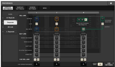
L Separate... When working with 2 operators, this setting allows the person controlling Bay L to work without interfering with the person operating Bay CR.
