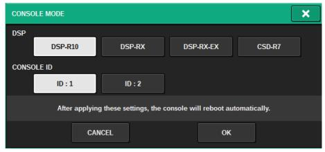
Specify separate CONSOLE IDs when using the system in dual console mode. The following functions are available only for the main console (ID1), but other functions are common to both.
