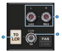
In the TO STEREO popup window, if the PAN/BALANCE select button is set to PAN, the L and R PAN knobs are displayed, allowing you to specify the panning of the signal. If you use the ST/LCR mode select button to select LCR, the LCR button (5) and CSR knob (6) are displayed. The LCR button turns on/off the signal that is sent from the channel to the STEREO bus, and the CSR knob specifies the level ratio between the signal that is sent to the STEREO A (L/R) bus and to the STEREO B (C) bus.
