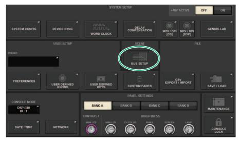
**2** Press the BUS SETUP button to open the BUS SETUP popup window.
