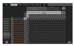
**3.** Use the knob in the upper-right corner to display the desired output jacks.
