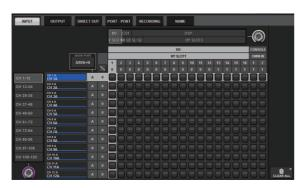
**3.** Use the knob in the upper-right corner to display the desired input jacks.
