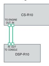
Use Ethernet cables to connect the TO ENGINE OUT/IN connectors on the control surface to the TO CONSOLE OUT/IN connectors on the DSP engine.
