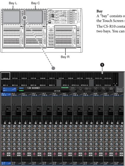
A "bay" consists of a group of 12 faders located across the Touch Screen section and the Channel Strip section. The CS-R10 contains three bays; the CS-R10-S contains two bays. You can control these bays independently.
