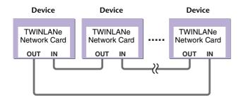
A TWINLANe network uses a ring topology, which provides redundancy in case of broken cables. If a cable in the network breaks down for some reason, the signal will be automatically re-routed and audio will flow without interruption. Even if a device in the network malfunctions, other working devices will be able to continue communicating.
