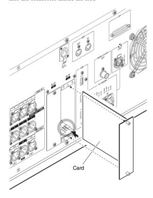
**4.** Fasten the card using the screws attached to the card.
