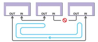
Even if a cable is severed at one point, the signal will be re-routed automatically and communication will continue without interruption.
