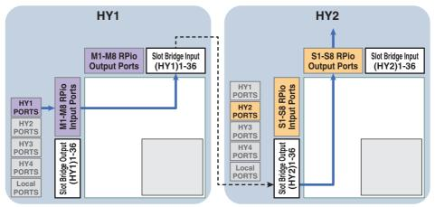
As an example here, we explain the procedure for patching from an RPio of a RIVAGE PM10 system's main network to an RPio of a sub network. In this case, multiple patches are required.
