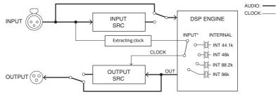
The input SRC converts the signal to the system clock of the RIVAGE PM series. The output SRC converts the signal to the specified internal clock source or to the same clock as the input of the same channel.
