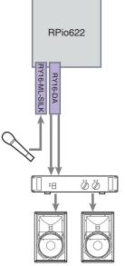
1 Analog input connection Connect a microphone or line-level component to the input jacks of the RY card (RY16-ML-SILK).
