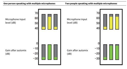
If one person speaks, that microphone's gain level will fade up instantly, while the other microphone gains will be reduced. If a different person speaks, the same effect will be obtained.
