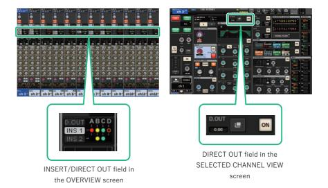
The "INSERT/D.OUT popup window (1CH)" (p.492)appears There are two types of INSERT/D.OUT popup window: 1CH and 12CH D. OUT.
