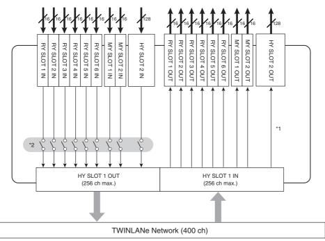
\*1) In mode 2, you can patch signals from the DSP engine to the HY SLOT 2 output via the TWINLANe network.
