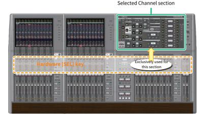
A [SEL] key is used to select the corresponding channel for the Selected Channel section (hardware). However, the [SEL] keys can also be linked to on-screen selected channels to assign channels to a DCA or mute group.
