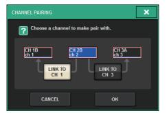
**3** Select the channel pairing direction, and then press the OK button.
