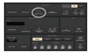
**1** Press the WORD CLOCK button in the SETUP screen.
