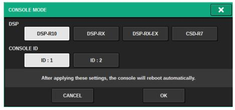
Specify separate CONSOLE IDs when using the system in dual console mode. The following functions are available only for the master console (ID1), but other functions are common to both.
