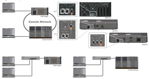
If you want to connect two computers to a DSP engine or control surface, use a switching hub to make connections.
