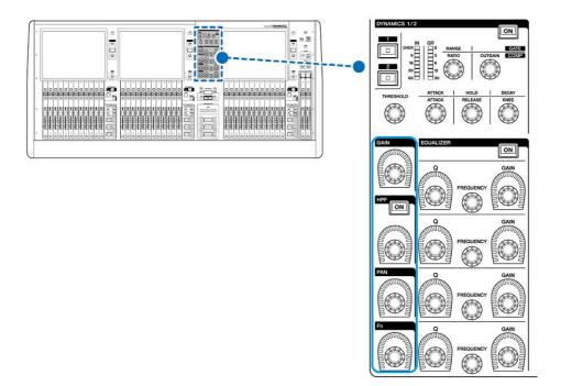
CH Parameter > Controlling GAIN via the Selected Channel section (CS-R5)
