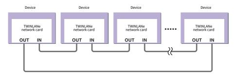
If a cable in the network breaks down for some reason, the signal will be automatically re-routed and audio will flow without interruption. Even if a device in the network malfunctions, other working devices will be able to continue communicating.
