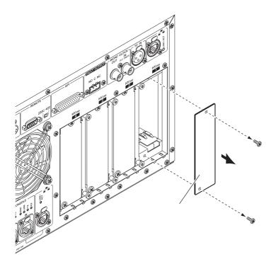
**3** Align both edges of the HY card with the guide rails inside the slot, and then insert the card into the slot with the card installation lever pressed down.
