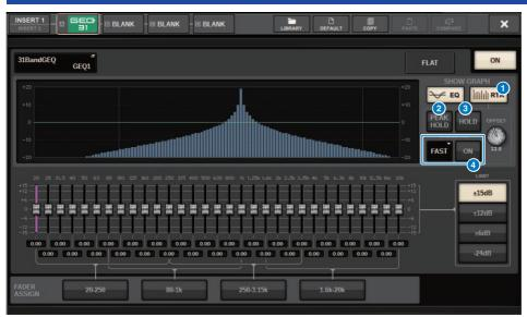
Press the rack container of the rack (which contains an inserted GEQ) to open the GEQ popup window.
