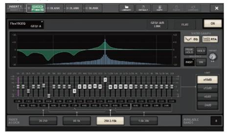
This window is the same as that for the 31BandGEQ, except that the AVAILABLE BANDS field is a real-time indication of the number of additional bands (maximum 15) that can be controlled for the current GEQ.
