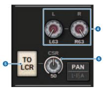
In the TO STEREO popup window, if the PAN/BALANCE select button is set to PAN, the L and R PAN knobs are shown, enabling you to specify the panning of the signal. If you use the ST/LCR mode select button to select LCR, the LCR button **(5)** and CSR knob **(6)** appear. The LCR button turns on/off the signal that is sent from the channel to the STEREO bus, and the CSR knob specifies the level ratio between the signal that is sent to the STEREO A (L/R) bus and to the STEREO B (C) bus.
