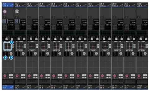
When the bus setting in BUS SETUP is set to surround mode, the OVERVIEW screen will appear as follows.
