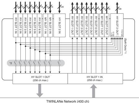
\*1) In mode 1, all input signals (total 128 channels) of the RY slots and MY slots are always split for output to the HY SLOT 2 output. The signal is output immediately after gain compensation.
