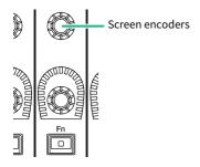
Screen encoders 1–12 are used to operate the knobs selected for operation in the touch screens. When you press to select a knob that can be controlled by the screen encoders, a thick frame appears around it. (Normally, a knob of this type corresponds to the screen encoder located immediately below that knob, allowing you to control up to twelve parameters simultaneously.)
