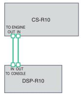
Use Ethernet cables to connect the TO ENGINE OUT/IN jacks of the control surface to the TO CONSOLE OUT/ IN jacks of the DSP engine.
