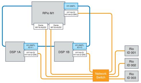
If the RPio622/222 is not connected, assign output patches from the Dante card (HY144-D, HY144-D-SRC, or Dante MY16-AUD card) that is installed on the control surface.
