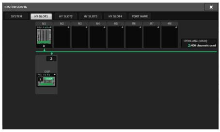
Press an I/O rack select button (in this case the M1 button). The I/O rack settings popup window will appear.
