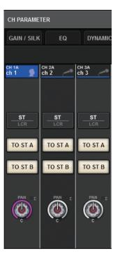
While pressing and holding down the [SHIFT] key, press the TO ST A/B button to access the PARAMETER SET (TO ST) popup window.
