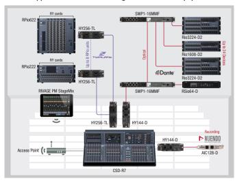
The Rio3224-D2 and Rio1608-D2 can be combined with previousgeneration I/O racks in CL/QL based systems, taking advantage of the simplicity and flexibility of Dante networking.
